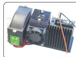
Powerful optical assembly with autosensing of cuvette or flowcell for proper positioning
